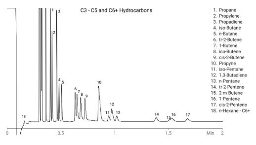
The Agilent 990 Micro GC is able to measure 17 different refinery gases in under two minutes.
